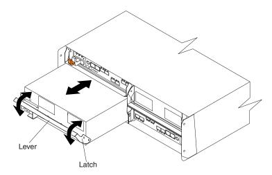
Figure 17. Removing a power supply and fan unit
